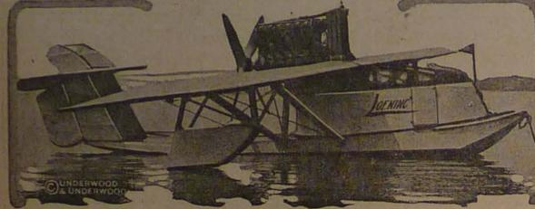
This machine is being built for Vincent Astor. The seating arrangement will be similar to that of a sedan motor car. With its 400 horsepower Liberty engine it will be capable of a speed of 135 miles an hour.
